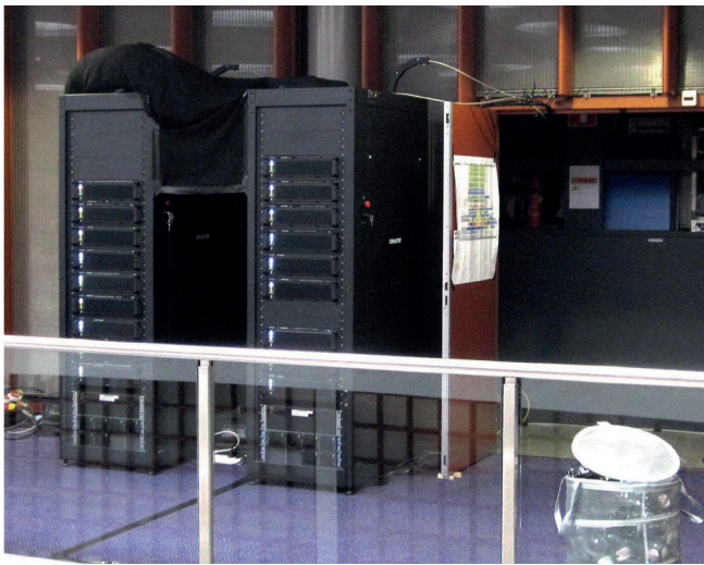
▲ Prototype RGB laser source by Christie Digital demonstrated at the IBC big screen theatre in Amsterdam 2012. Installed just outside of the projection booth, the thin white cables visible above the door are glass fibers carrying the laser light from this light source towards the DLP projectors in the booth.
